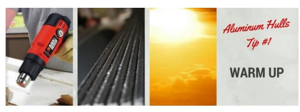
• Lay the KeelShield out in the direct, warm sun for 30 minutes to make the material as flexible as possible to form around the keel and any ribs or protrusions. You can also use a hairdryer to accomplish this.
