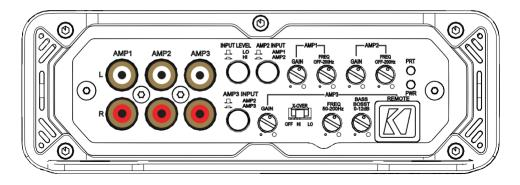
**Automatic Turn-On Selection:** The KMA series offers two different automatic turn-on modes that can be selected on the end panel; +12V and DC Offset. Using the DC Offset mode causes the REM wire to have +12V out for turning on additional amplifiers.
