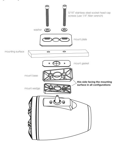
**Step 3:** Align the mounting hardware and begin to fasten the bolts. Use the mount gasket in all mounting configurations to ensure a water-resistant seal and to protect from cosmetic damage. You may also install an additional mount gasket between the mount plate and mounting surface. Make certain the wires have been fully extended through the mounting hardware and mounting surface before you finish tightening the bolts.
