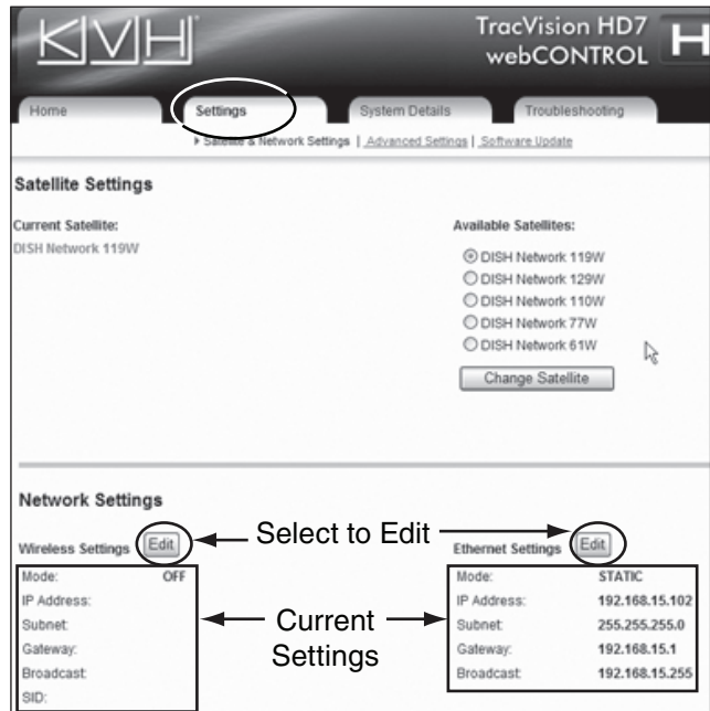
Figure 31 Network Settings on the Web Interface
