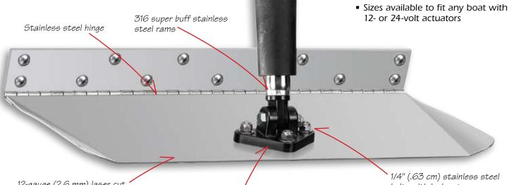
12-gauge (2.6 mm) laser cut stainless steel trim tab blades
