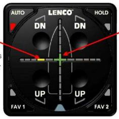
THE GREEN CENTER LED REMAINS ILLUMINATE TO INDICATE THAT THE BOAT'S **CURRENT PITCH POSITION** STILL MATCHES THE AUTO GLIDE'S **HOME PITCH DEFAULT POSITION**.
