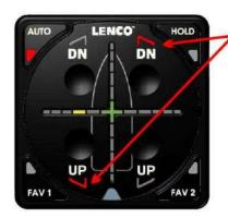
TO MAKE A ROLL CORRECTION, THE AUTO GLIDE MOVES BOTH THE PORT AND STARBOARD TRIM TABS AT THE SAME AMOUNT, BUT IN THE OPPOSITE DIRECTION
