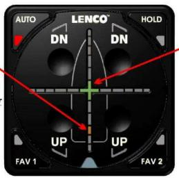
THE GREEN CENTER LED REMAINS ILLUMINATE TO INDICATE THAT THE BOAT'S CURRENT ROLL POSITION STILL MATCHES THE AUTO GLIDE'S HOME ROLL DEFAULT POSITION.
