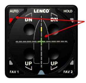
THE "AUTO" AUTOMATIC SETTING LED INDICATOR ILLUMINATES ONCE THE AUTO GLIDE HAS VERIFIED IT HAS ALL OF THE REQUIRED ENGINE AND GPS DATA PLUS THE HOME ROLL AND PITCH DEFAULT POSITIONS HAVE BEEN STORED.
