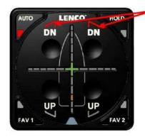
TO MAKE A PITCH CORRECTION, THE AUTO GLIDE MOVES BOTH TABS UP OR DOWN AT THE SAME TIME.
