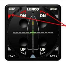
PRESS THE SELECTED AUTO BUTTON TO OVER-RIDE ROUGH WATER HOLE SHOT MODE. THE AUTO GLIDE FULLY DEPLOYS THE TRIM TABS, EVEN THOUGH IT SENSES ROUGH SEA CONDITIONS:
