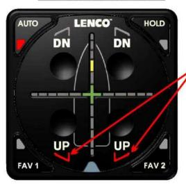
IF YOUR BOAT HAS MERCURY DTS DIGITAL SHIFT OR NMEA 2000 DIGITAL SHIFT SYSTEMS, THE AUTO GLIDE *FULLY RETRACTS THE TRIM TABS* WHEN YOU SHIFT INTO REVERSE WHILE THE AUTO GLIDE IS IN *HOLE SHOT MODE*.
