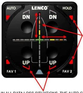
WHEN ENGINE DATA LOSS OCCURS, THE AUTO GLIDE WILL FLASH THE OUTSIDE FOUR (4) AUTOMATIC SETTING LED INDICATORS AND THE CROSSHAIR LED INDICATORS WILL SCROLL FROM THE CENTER TO THE TWELVE O'CLOCK POSITION AND FROM THE CENTER TO THE THREE O'CLOCK POSITION.
