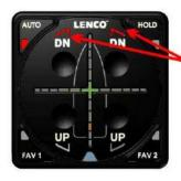
DURING AN AUTOMATIC BOAT CONTROL DECISION, THE AUTO GLIDE EXTENDS BOTH ACTUATORS TO CORRECT FOR A PITCH ANGLE THAT IS ABOVE THE HOME PITCH POSITION.
