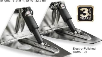
Blades are constructed of Electro-Polished 7 gauge (4.6 mm) laser cut 304 stainless steel with heavy duty hinge with 3/8" (9.5 mm) diameter hinge pin. Full transom back plate with mechanical strain-relief cable seals, welded on stainless steel upper & adjustable lower actuator mounting brackets, 3/8" (9.5 mm) stainless steel mounting bolts. 3.75" (9.5 cm) sacrificial anodes installed.
