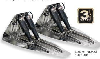
Blades are constructed of Electro-Polished 7 gauge (4.6 mm) laser cut 304 stainless steel, heavy duty hinge with 3/8" (9.5 mm) diameter hinge pin. Full transom back plate with mechanical strain-relief cable seals, welded on stainless steel upper & adjustable lower actuator mounting brackets, 3/8" (9.5 mm) stainless steel mounting bolts. 3.75" (9.5 cm) sacrificial anodes installed.
