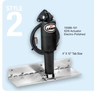
Blades are constructed of 12 gauge (2.7 mm) laser cut 304 stainless steel with a folded over trailing edge for safety, welded on lower mounting brackets & 1/8" (3.2 mm) diameter hinge pin. High impact corrosion proof upper mounting brackets with mechanical cable gland seal.
