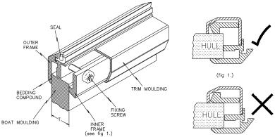
Typical installation cross section
