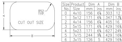
It is essential that the outer frame is placed squarely on the deck opening. When fitting a number of portlights it is advisable to prepare a template.
