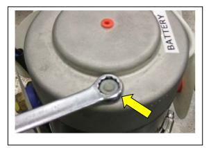
2. Use a spanner to remove the cover retaining nuts, then lift off the cover, being careful not to damage any wires.
