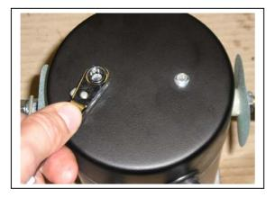
2. Use a spanner to remove the cover retaining screws, then lift off the cover, being careful not to damage any wires.
