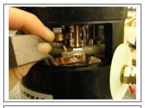
5. Totally remove the old brush from the housing replacing with the new one. Replace the parts removed during stages 2 to 4 in reverse order.
