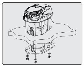
Pass all the studs through the deck and fit the metal clamping plate to the underside of the deck and secure the unit with the fixings provided.
