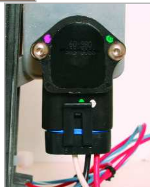
ETPAS dual redundancy pot for throttle lever
