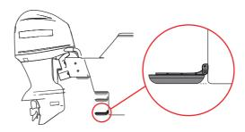
The transducer can be mounted on a transom bracket. With this mounting option the transducer can be in the water when you are on plane, or can be mounted so it is only in the water when you are moving at trolling speed.
