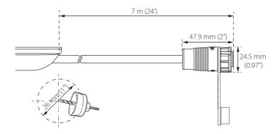
A 26mm (1") diameter hole is recommended for cable clearance.
