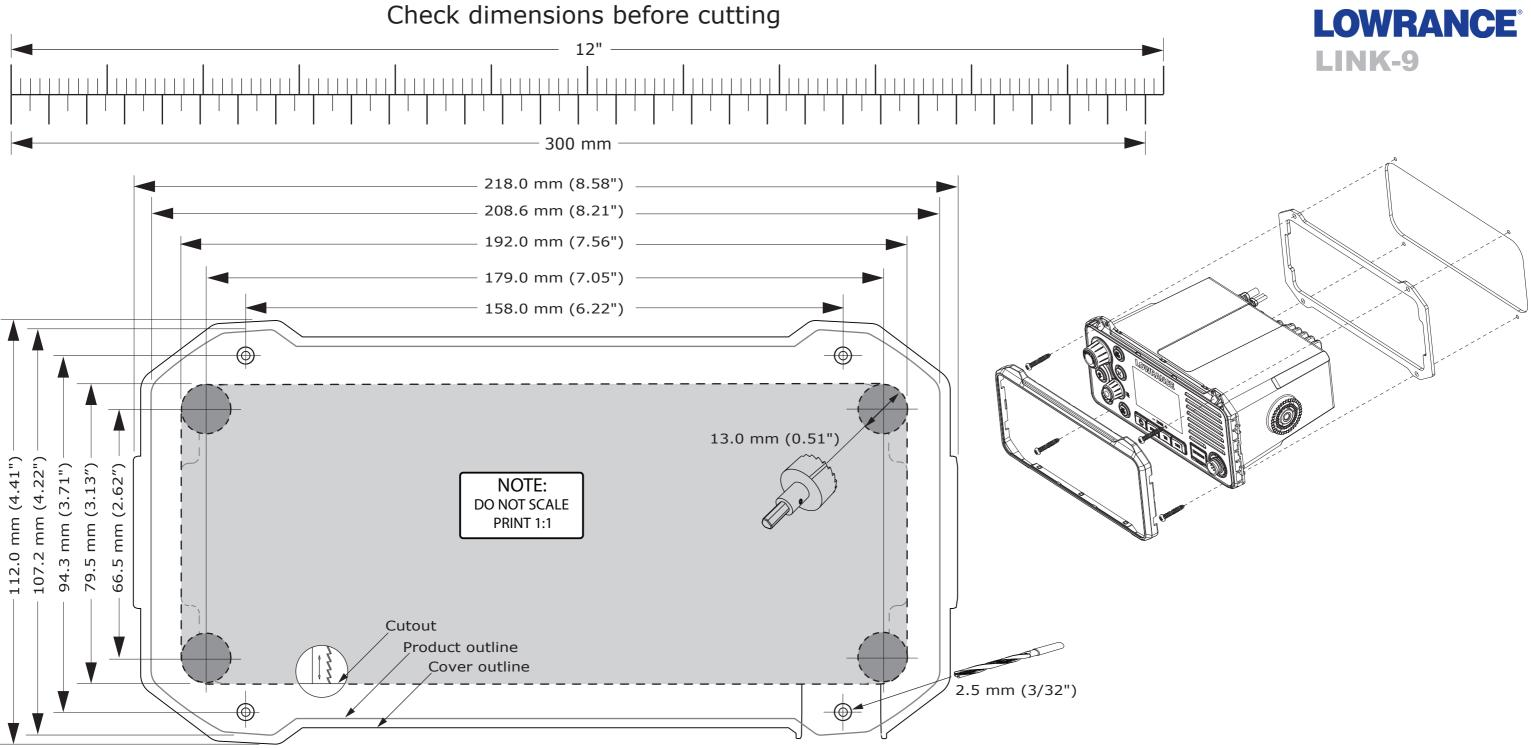
IMPORTANT. Do not use this template if it has been rescaled by copying or printing. If this is not the original, or is a print from a file, please check the dimension lines above are to scale before use.
