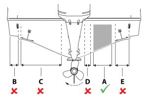
Mirror the example if your boat has a counterclockwise propeller rotation.
