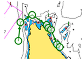
Result after automatic routing
