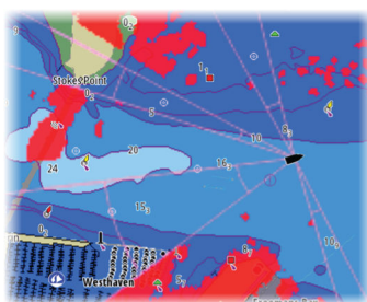
Radar overlay on a chart
