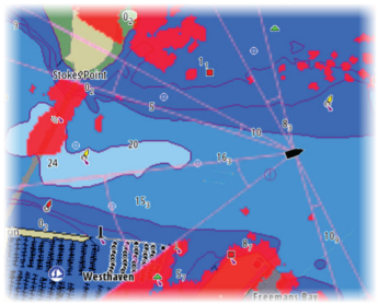
Radar overlay on a chart
