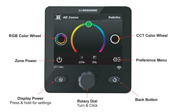
The Lumi-Link Display is very easy to use, It is a touch screen device but can also be used with the rotary dial. Use the rotary dial to move the cursor around the screen, pressing the rotary dial will select the icon/slider bar or text that is highlighted.
