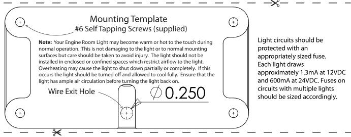
Thank you for purchasing the Engine Room Light. This light utilizes Lumitec's proprietary technology to cast a broad, even light over a wide area in a color optimized for easy viewing and reduced eye fatigue.
