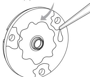
Lights may be painted, but ONLY with paints explicitly intended for aluminum substrates. Anti-fouling paints which do not explicitly state that they are safe for aluminum substrates can be damaging to the BayBlaze light, and should not be used on surfaces within 1" (2.5cm) of the light.
