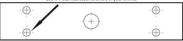
Center hole can be used for a 1/2" center bolt or wire exit hole.
