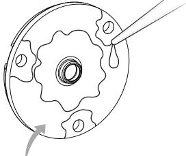
Thoroughly coat the entire back surface surrounding the mounting stem and screw holes with polyurethane marine sealant.
