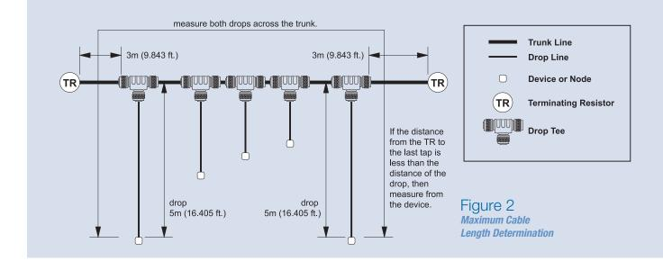
opposed to Micro cable (4 amps). Mini cable has an outside diameter in the range from 0.41 to 0.49 inches. Its maximum installed bend radius is 7x the cable diameter. You can also use this type of cable for drop lines.
