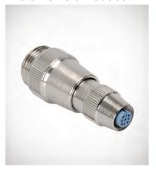
The reducer is used to change from a Mini cable to Micro or Mid cable. For example, one end of the network might be terminated at the top of the mast but it may not be desireable to run a Mini trunk cable up the mast. In this case, you can switch over to Micro or Mid cable at the base of the mast using the reducer and continue up the mast with Micro or Mid cable.
