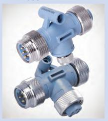
A Tee is used to tap into the trunk line for adding a drop connection. Two Mini Tees are available: 1) a Mini Tee with Mini connectors for the trunk and drop lines, and 2) a Mini/Micro Tee with Mini connectors for the trunk lines and a Micro connector for the drop line.
