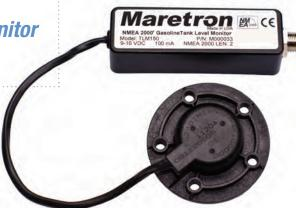
The TLM150 is mounted directly to the top of tanks using the industry standard SAE J1810 5-hole mounting pattern. The TLM150 can also be mounted to tanks with threaded tank openings using optional adapters that include both a 1.5" NPT and a 1.25" BSP adapter. The other important optional accessory for the TLM150 is the focus tube to permit use on boats with planing hulls, which is required if the vessel spends a significant amount of time with the bow pitched up.
