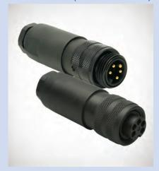
Field-attachable connectors allow you to make field connections to bulk cable. The color-coded screw terminals match the individual wire colors found within the bulk cables for error-free field installation.
