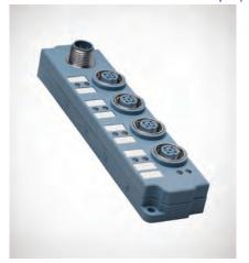
Multiport boxes allow several drop cables to be consolidated and connected back to the trunk, which eliminates the need to have numerous tees connected near a single point. Multiport boxes connect back to the trunk through a double-ended cordset and Tee.
