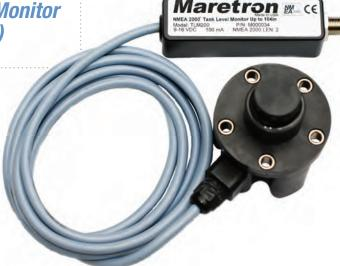
The TLM200 is mounted directly to the top of tanks using the industry standard SAE J1810 5-hole mounting pattern. The TLM200 can also be mounted to tanks with threaded tank openings using the optional 1.5" NPT adapter.
