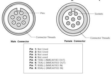
Connect the other end of the cable consisting of individual wires using recommended practices for installing NMEA 0183 products. Please note that NMEA 0183 does not have a standard for connectors and the customer/installer should contact the manufacturer of the equipment to which the compass is being connected for information on how to properly connect the device to the compass. The individual wires found within the cable have the following color coding:
