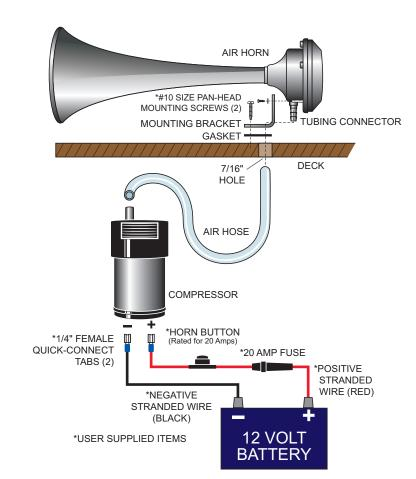
fitting and pressing it up about 1/2". Reinstall the horn to the mounting bracket with the two phillips-head screws. Use a small amount of silicone sealant to seal any gaps between the air hose and opening hole to prevent water from leaking inside. Make sure not to squeeze the air hose as this will impede the air flow.
