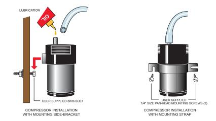
onto the compressor by sliding it over the air port opening. Be sure there are no kinks in the air hose that will impede air flow.
