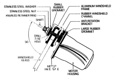
the outside of the frame followed by the washer and nut. Use a 14 mm or small adjustable wrench to tighten the nut snugly. Do not over-tighten. Install the knurled retainer ring. Be sure the rubber grommets are on both sides of the frame.
