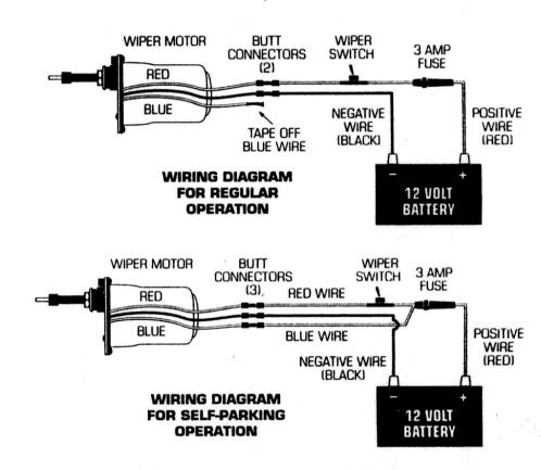
Strip 1/4" of insulation from each of the wires on the motor. Attach wiring together with crimp-on butt connectors and seal with electrical tape. If the blue wire is not used, seal off and insulate the end of the wire with electrical tape.
