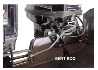
Typical installation options are shown here. It may be necessary to bend the threaded rod to fit your application
