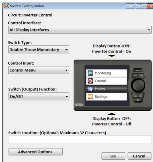
3. Under Circuit Loads select the MasterBus Event Source virtual load we created above in the Loads section (e.g. "Inverter Control").
