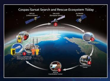
All you need to access this free of charge ecosystem is an emergency beacon that operates on the 406 MHz frequency.
