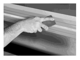
\*To keep your PontoonGuard looking new, clean with mild soap and water. If you wish to reapply any metal protectants or clean the tubes using acid based or chemical cleaners, the PontoonGuard must be masked to protect the finish and reflective film.
