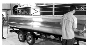
Measure the length of the pontoon tube. If the PontoonGuard is too long, trim the PontoonGuard with a utility knife on the rear squared edge for a precise fit.
