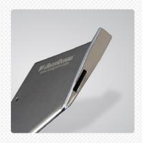
This 3mm thickened lower plate will withstand damage or abrasion from hidden rocks and debris or accidental ramp dragging. The Megaware SkegGuard® conforms to your lower unit to insure there is no discernible drag or compromise in performance. A drain hole keeps water from collecting and remaining stagnant.
