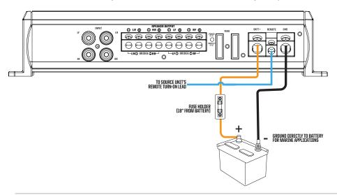
\*NOTE: Seven inches is the standard distance under U.S. Coast Guard CFR33 for placement of fuses or breakers as required by law for new boat manufacturing. It is recommended that you adhere to this standard in an installation. Not adhering to this regulation puts the safety of boat passengers at risk in the event of a power wire shirt circuit
