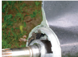
The shaft taper takes forward thrust from the thrust washer. Without a forward thrust washer, the gearcase takes the forward thrust as the propeller will continue to move forward on the shaft, causing severe damage to the gearcase.
