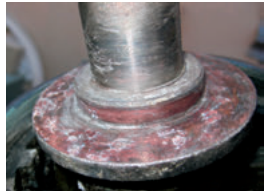
Over time, the forward thrust washer may appear as part of the propeller shaft. It is still necessary to remove the thrust washer when installing an XHS propeller.
