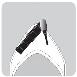
Position the Bowmount close to the centerline of the boat and in an area free of obstructions.
