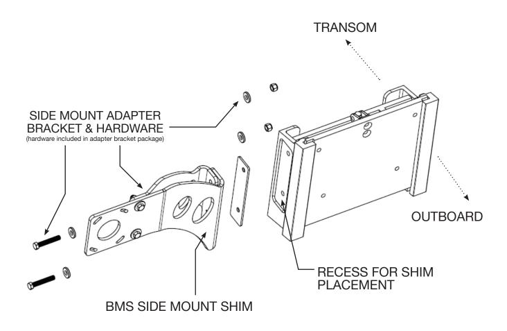
**MOUNTING EXAMPLE:** 6" SETBACK, PORT, JACK PLATE MOUNTED ADAPTER BRACKET ON BOBS MACHINE SHOP JACK PLATE USING SIDE MOUNT SHIM.
