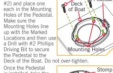
is installed, take the Wireless Stomp Switch and reattach it to the Pedestal. Make sure the Notch on the Pedestal is aligned and then click the Tab in place so that the Wireless Stomp Switch is fully seated into the Pedestal on the Deck of the Boat.
