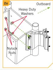
**NOTICE:** To prevent seizing of the stainless steel hardware, do not use high speed installation tools. Applying an anti-seize may help prevent seizing.
