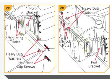
**NOTICE:** To prevent seizing of the stainless steel hardware, do not use high speed installation tools. Applying an anti-seize may help prevent seizing.
