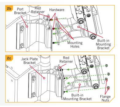
d. With the Flange Nuts in place, pull the Red Retainer out to release the hardware. There are handles on each side of the Red Retainer that can be used to grasp each half. When pulling the Red Retainer, grasp each side and pull so that the Red Retainer breaks at the center and releases the hardware.
