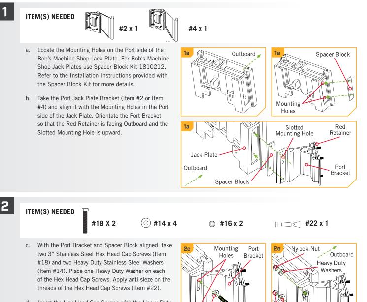
d. Insert the Hex Head Cap Screws with the Heavy Duty Washers in place through the Mounting Holes in the Port Bracket and Spacer Block and into the Holes on
