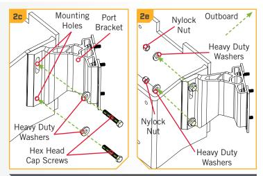
**NOTICE:** To prevent seizing of the stainless steel hardware, do not use high speed installation tools. Applying an anti-seize may help prevent seizing.
