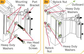
**NOTICE:** To prevent seizing of the stainless steel hardware, do not use high speed installation tools. Applying an anti-seize may help prevent seizing.
