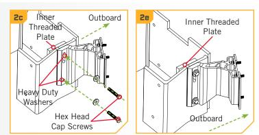
**NOTICE:** To prevent seizing of the stainless steel hardware, do not use high speed installation tools. Applying an anti-seize may help prevent seizing.
