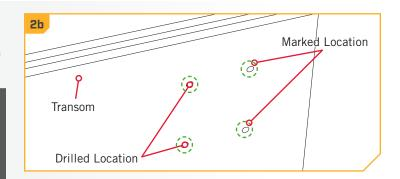
**NOTICE:** When drilling the marked holes, make sure that the drill bit is perpendicular to the Transom/Stern of the boat and that the holes are being drilled straight. Not drilling the holes straight will give the mounting hardware a poor fit.
