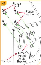
**NOTICE:** An alternate option is to mount the bracket, by passing the Hex Head Cap Screw with the Fender Washer from the inside of the transom to the outside. Pass the Screws into the Drilled Locations. Then pass them into the Direct Mount Angle Bracket. Secure on the outside of the boat with the Flat Washer and Flange Nut.
