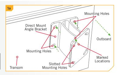
b. Double check that the mounting location is clear to drill holes and then use a Drill with a 7/16" Drill Bit to drill through the Transom/Stern of the boat on the marked locations.
