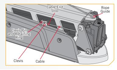
e. Pull on the Cable Handle until the Clevis slides into the opening between the Latch Bar and Latch/Strap Rope Pull Bracket.
