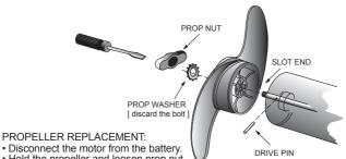
· Disconnect the motor from the battery.
