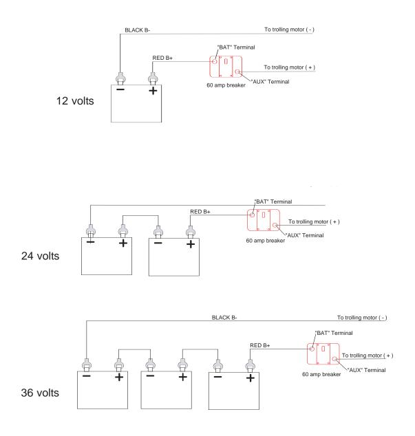
**NOTE:** The 24 / 36 volt diagrams shown here show a series link being made at the batteries. Some installations will have the series link made at the trolling motor plug or plug receptacle.
