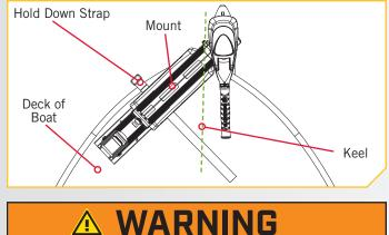
When raising or lowering motor and tilting motor, keep fingers clear of all hinge and pivot points and all moving parts.
