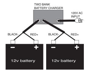
NOTE: If batteries are connected in series for 12/24 - 24V, the series connection wire should be left in place during charging.
