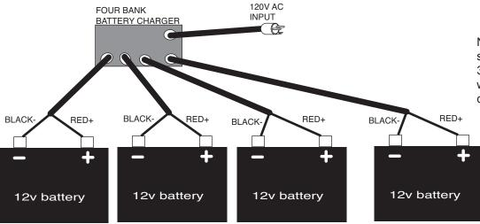
NOTE: If batteries are connected in series for 12/24 - 24 - 24/36 - 36V-36/48 - 48v, the series connection wire should be left in place during charging.
