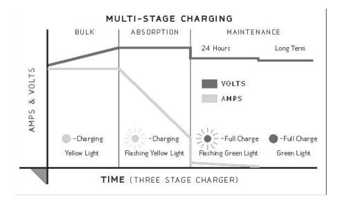
indicate the battery is in Maintenance Mode and ready to use. After 24 hours, the charger automatically turns off and a GREEN light is lit for each bank to indicate the battery is in long term Maintenance Mode and ready to use. The charger will automatically turn on when the battery voltage drops below 12.6V.
