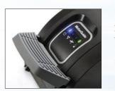
LED status indicators help you monitor four key motor functions at a glance, including three levels of battery life.
