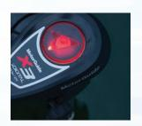
Foot control models feature a lighted steering indicator illuminated with LEDs. (Digital models only)
