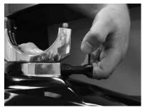
10. Tighten the locking knob by hand. Next use an 18mm open end wrench to tighten down the lock knob so it wont move. Using the 18mm wrench will ensure enough torque is applied to keep the unit from loosening.
