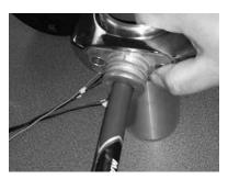
3 Drill a 5/6" hole where the mark was made. The speaker wire/dome light and LED logo power wire will be passed through this hole. Place a grommet in the drilled hole so the wire will not be damaged by the sharp edge of the pipe.
