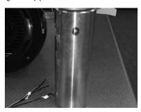
Pull the wires through the bar that the WET8CWB is being mounted to. Pull the wire harness wire through the bottom of the bracket. The white connector should be on the bottom side of the bottom bracket.
