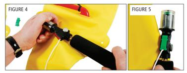
Step 4 - Check to be sure service indicator is green inside clear cap and the green indicator clip is firmly attached to the activation lever (Fig. 5).
