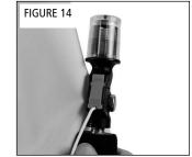
Step 4 - Check to be sure service indicator is green inside clear cap and the green indicator clip is firmly attached to the activation lever (Fig. 14).
