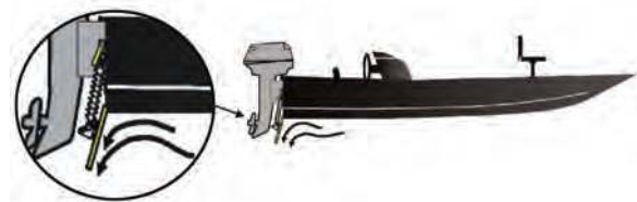
WHEN DOWN, THE PROROLLER SMART TABS ACT AS BRAKES TO REDUCE TROLLING SPEEDS BY UP TO 35% WITHOUT LOSING STEERING CONTROL.
