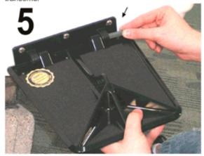
Attach the Plate: Align the plate & hinge holes, and use the 3/8" diameter 'snap & lock' pins to secure the plate to the hinge. Push the pins in until the head is flush. This may take some effort.
