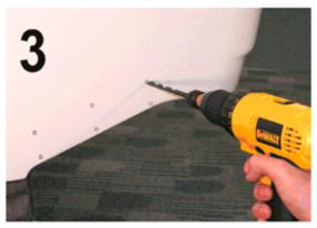
**Drill the holes:** Use a 7/32" drill bit for Fiberglass transoms and a 3/16" drill bit for aluminum and wood transoms.
